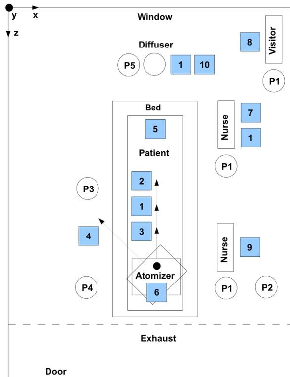
Figure 1. Ventilation test setup
